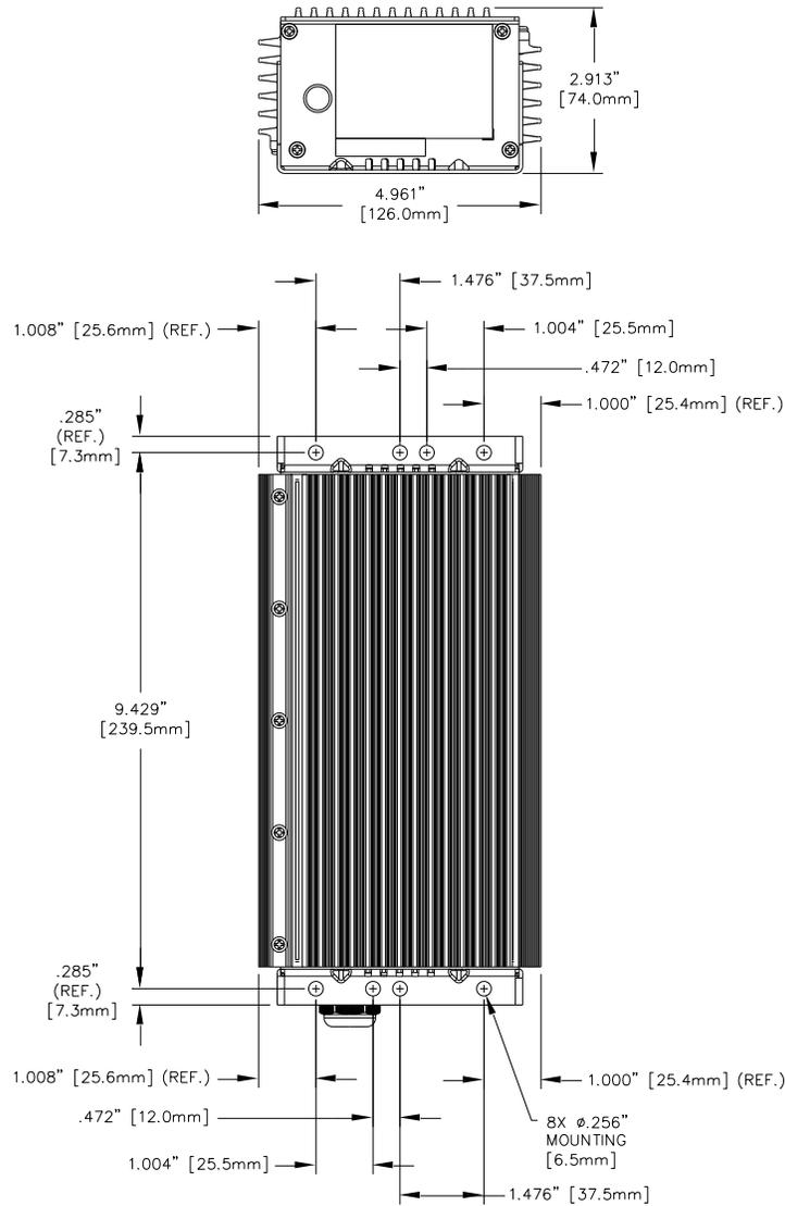
**Figure 2-1: Charger Dimensions and Mounting Slot Locations**
