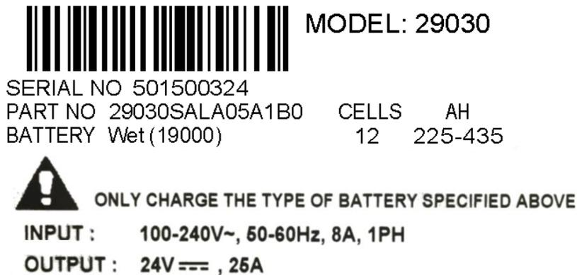
Document any configuration or settings changes that are made by marking the ratings label on your charger or on an additional label or tag attached to your charger.
