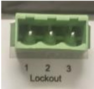
Figure 8-1 charger lockout relay terminals. 1=NC, 2=COM, 3=NO
